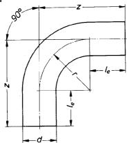
Designation of a B2 pipe bend with a 90° angle and external pipe diameter  $d = 400 \, \text{mm}$  of pipe series 3 and
